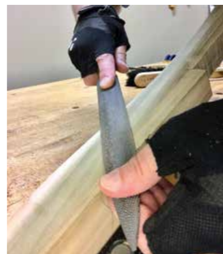
Use a rasp to smooth the blank to your layout lines...
