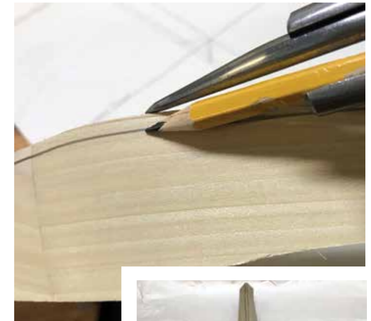
The centre aris should be straight when initial shaping is complete
