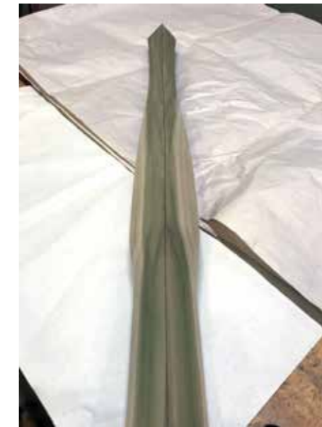
The centre aris should be straight when initial shaping is complete
