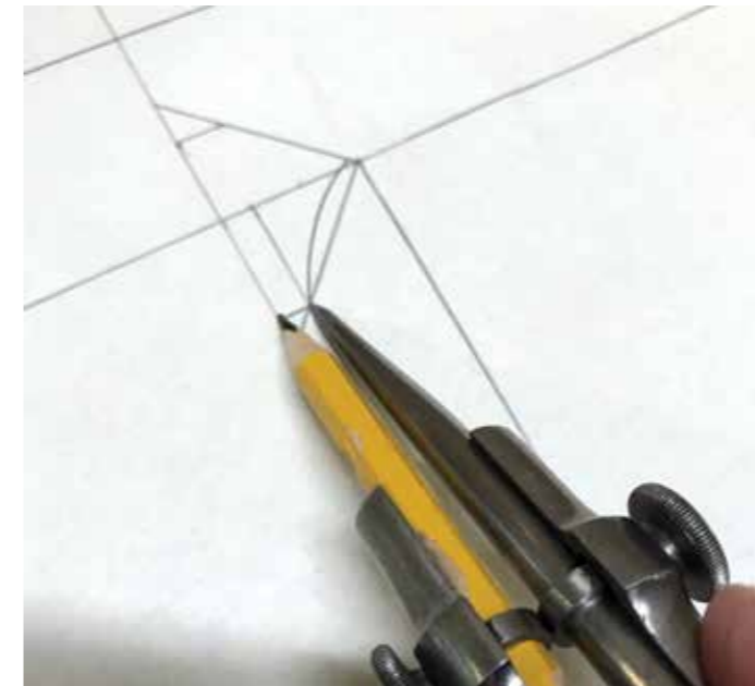
Above and right: marking the chamfer
