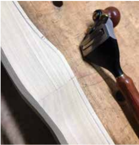
Pencil layout lines a few centimetres away from the rear arrises on the side faces of the leg. I use a Veritas pullshave to remove material quickly, but any convex spokeshave will work
