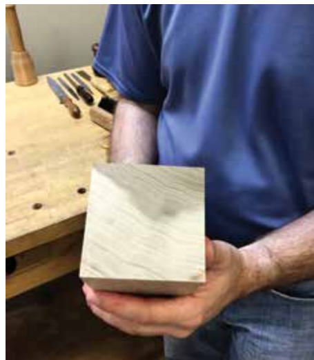
Choose rift sawn stock, where the growth rings run diagonal across the end grain of the blank, for legs where the solid wood will show
