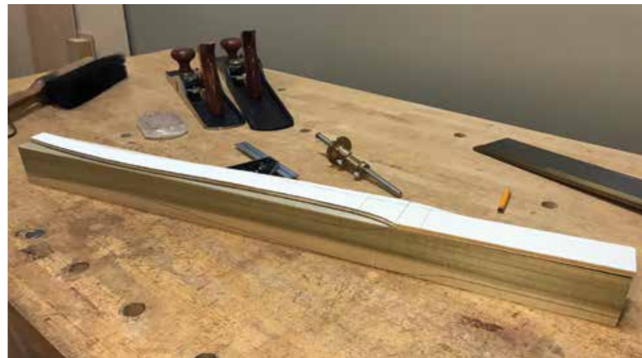
Carefully align and trace the side view drawing to the reference surfaces of the leg blank. Keep the 'rear' side of the template against the aris of the reference surfaces
