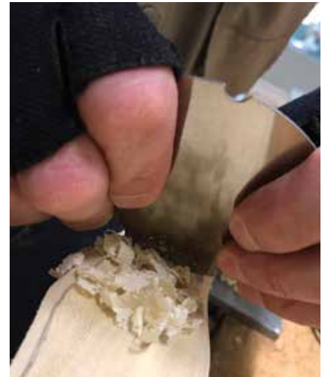
A convex scraper refines the surface
